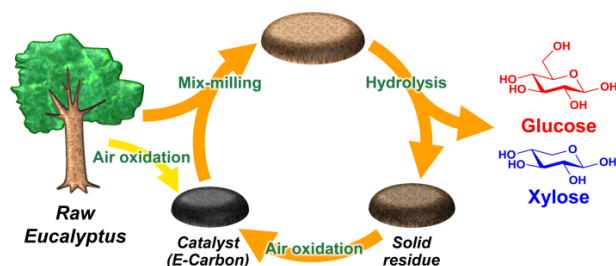
Fig. 3 Hydrolysis of woody biomass by a biomass-derived reusable carbon catalyst.
